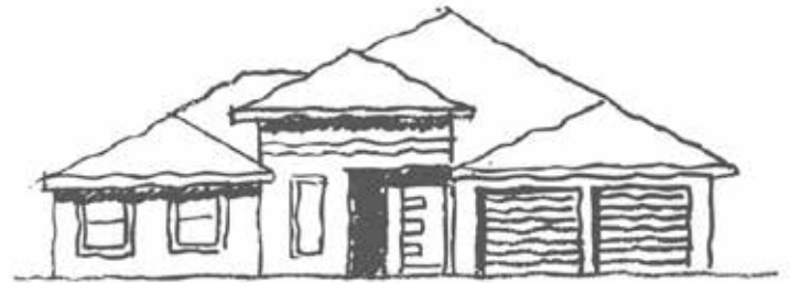
Figure 3.1.1 Primary Frontage Presentation Primary Frontage Presentation incorporating design elements including a recessed entry porch, varied setbacks, varied roof forms, well proportioned windows and a split garage.
