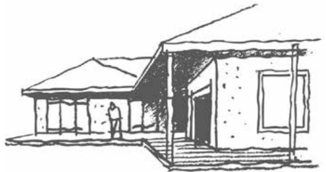
Figure 3.2.2 Design for Climate Patios provide covered outdoor living areas as well as providing shaded openings and allowing for covered clothes drying
