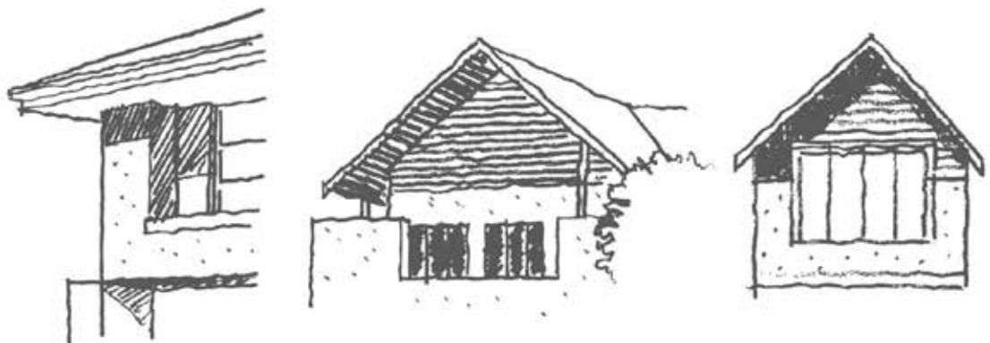
Figure 3.1.6 Roof form Incorporate roof forms with eaves to provide shade to windows and balconies and create an interesting and attractive appearance.
