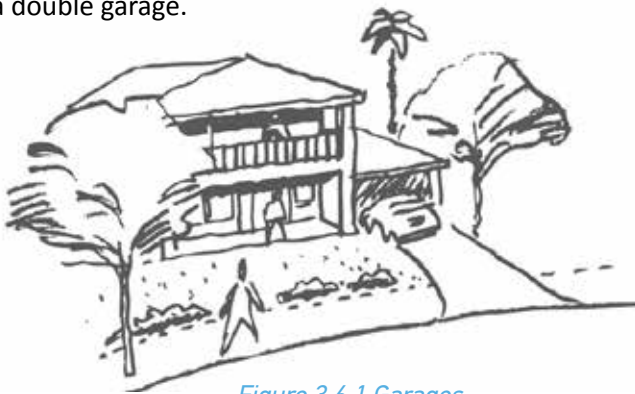
Figure 3.6.1 Garages Incorporate garages into the design of the dwelling and minimise their impact on the street by minimising the driveway width and incorporating landscaping on both sides
